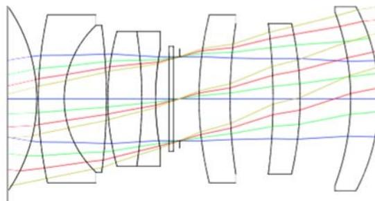
Figure 10 – Part of the optical design of the fisheye lens with in the center the pupil location (diaphragm) and new chopper (visible as plan plate at left side of pupil).
